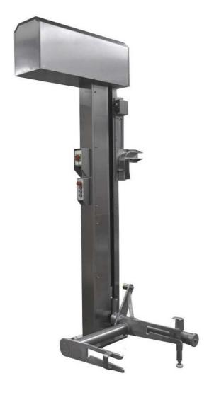
Lifting- tipping device 2550-3050 mm Rigth side, stationary 90° rotated fork
