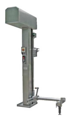
Lifting / tipping 1050-1550 mm for 120 L eurobins DIN9797 rigth side, stationary
