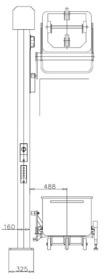
3 x 400/ 50 Hz 24 V AC 0.75 kW IP 65 5 m/min 937 mm 325 mm 1.013mm 4.490 mm
