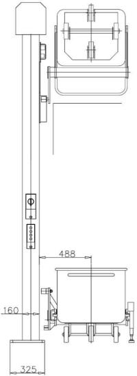
3 x 400/ 50 Hz 24 V AC 0.75 kW IP 65 5 m/min 937 mm 325 mm 1.013mm 4.990 mm 576 4990 260 4050 445 937
