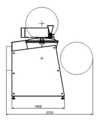
\*operating pressure can be reduced to 3 bars. The basic machine consists of 80 L drum AISI 316, without heat exchange- coat (with steam), with thermoisolation, cutter knife -3 pcs. 5 mm, stirrer 70 r/Min., programming possibilities, aluminium pneumatic cylinder, speed motor -22 kW.
